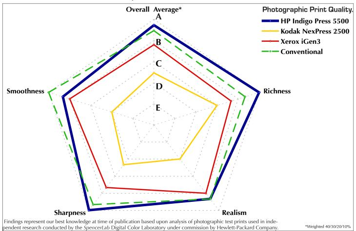
HP Indigo press 5500 prints displayed well saturated, vibrant color that did not overpower Realism. The optical density of black was the best of the competitive group at over 2.5 ODU (less than 3 CIE  $L^*$ ). This earned a relative grade of "A". In comparison:
